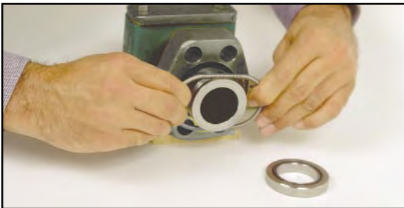
Step 3: Retain ring is sprung over the pipe's outside diameter nesting in the annular groove.
