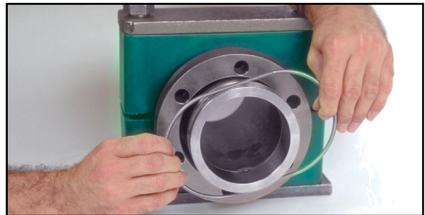
Step 4: Slip flange onto the pipe. Retain ring is sprung over the pipe adapter's outside diameter nesting in the groove.
