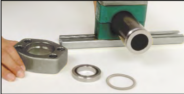
Step 1: Pipe supplied with butt end machined along with an annular groove on the outside diameter.
