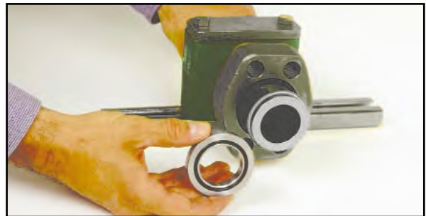
Step 4: Select the correct 'o' ring spacer style. The 'o' ring provides a seal against the butt end of the pipe.
