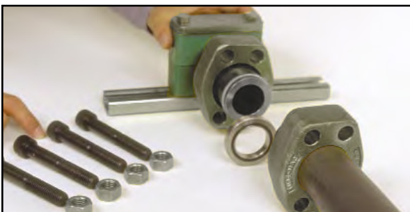
Step 5: Select the required bolting hardware from Section R of this catalogue. Carefully place the 'o' ring spacer in between the pipe ends. Slide the flanges forward and the 'o' ring seal retainer becomes captive within the flanges.
