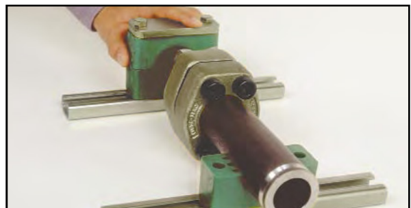
Step 6: Tighten bolts to the torque values specified. Always tighten bolts in a cross-over sequence and ensure that the flanges are parallel.
