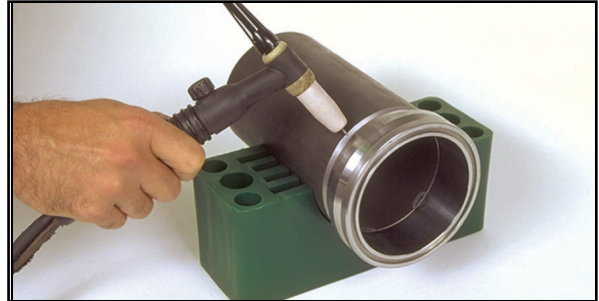
Step 2: Select the correct low pressure retain ring butt weld adapter to suit the pipe size. Weld the root pass with tig, then use #7018 welding stick for the filler and weld cap.
