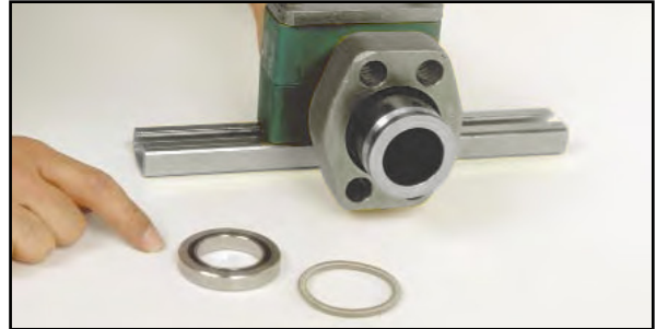
Step 2: Slip flange onto the pipe.
