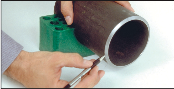
Step 1: Cut pipe end square, and bevel for butt weld.
