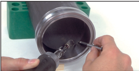
Step 3: Grind the weld on the inside of the pipe using a pencil type grinder. Clean the inside of the pipe after grinding.
